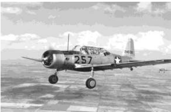
The BT-13 Valiant was a stellar trainer aircraft used for basic flight training and for blind instrument training throughout World War II. (www.militaryfactory.com)
